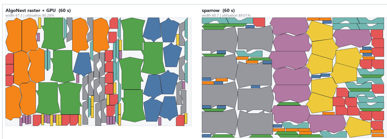
Figure 2. shirts — 99 pieces, 60 s, same machine. Left: our raster engine, 80.28%. Right: sparrow, 89.01%. Note how sparrow interlocks neighbouring shapes and leaves far less white space; our constructive decoder places each part once and never revisits it.
